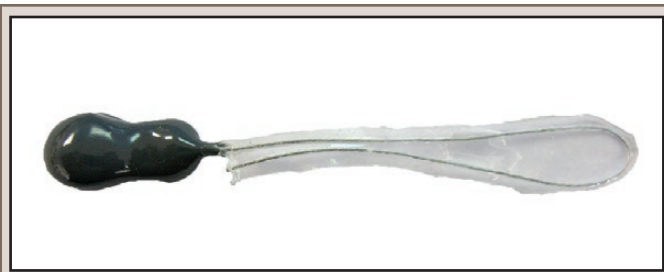
FIG. 1. Holohil BD-2 radio transmitter with a 10-cm whip antenna looped and encased in a thin layer of clear silicone. Transmitter length varies due to varying loop lengths to fit the coelomic cavity of individual animals.
