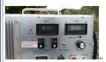
Example of the older style of electrofishing control box capable of generating 40 amps. While great in typical systems, this unit struggles in high conductivity systems.
